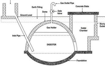
Fig. 4: Schematic diagram of a Deenabandhu biogas plant
