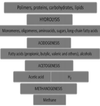
Fig. 1- Typical representation of anaerobic of complex substrates to biogas
